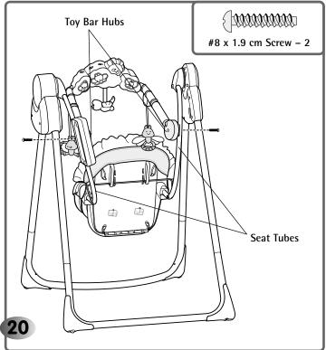
• Fit the toybar hubs to the seat tubes.
